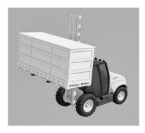
Crates must be lifted with a forklift or a crane.
