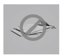
If the panels are stored horizontally, panels must be stored on a flat surface. All corners should be in contact with the surface. Panels should not be stored on the edge of the platform.
