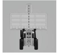
Operators must ensure that the crates are fully supported and balanced before lifting.
